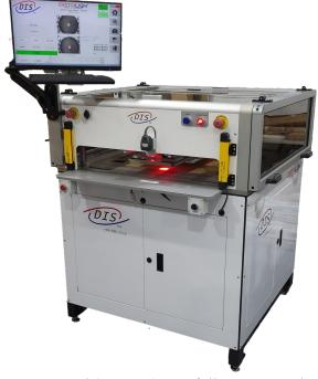
The Optical Lay-up Station Manual (OLS-M), is a fully automated system including automated weld bars and heads for different panel sizes and welding positions. This system is capable of handling a range of job sizes from prototype runs to small volume multi stackup production runs.
